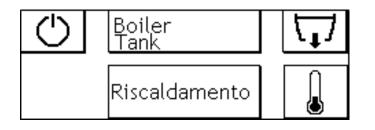
After filling the heating screen appears. The water of the boiler and the water of the tank is heated to the minimum operating temperatures. The temperatures are shown in the centre of the display.
