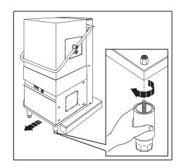
4. Slide the machine further off the pallet until the first side is standing on its own two feet and the other is still supported by the pallet, so that the two remaining holes are free; then proceed as explained above.
